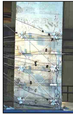
Figure 3.16 (F1 & F2) Flexural and Longitudinal Cracking
