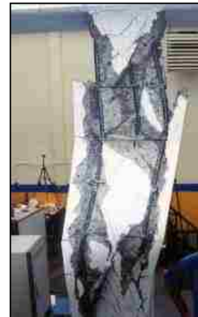
Figure 3.27 (S3.3) Longitudinal Bar Buckling
