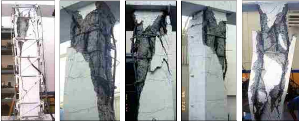
Figures 3.87, 3.88, 3.89, 3.90, and 3.91 Longitudinal bar buckling: experimental damage (Sezen 2002)
